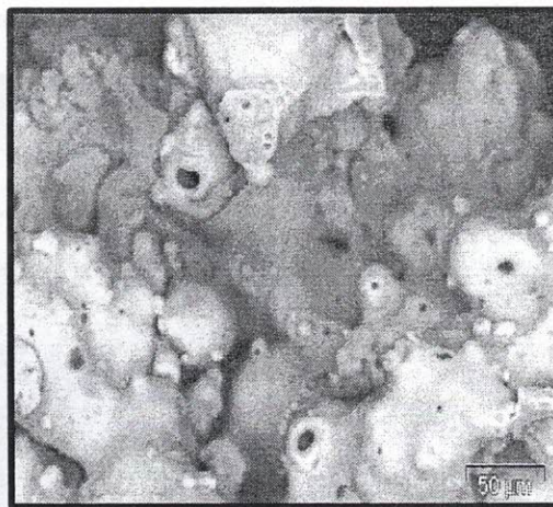
DIC treated skimmed milk powder P= 2.3 bar , W=8 % DB, t= 16 sec
